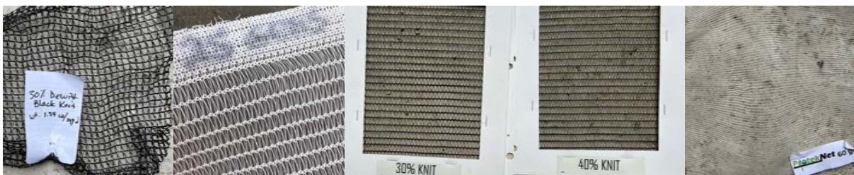
Figure 2. Mesh exclusion materials tested: DeWitt 30% black, Gintec 25g white, Gintec 30% black, Gintec 40% black, and ProtekNet 60g white.
