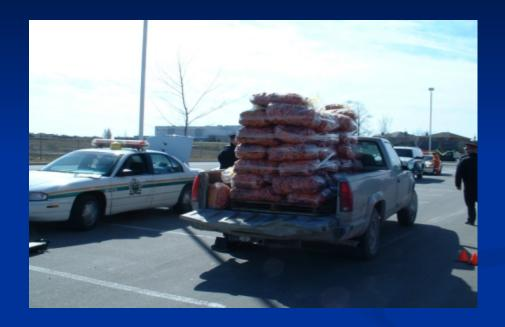
No person shall operate or permit to be operated upon a highway a motor vehicle/commercial motor vehicle that carries a load or draws a vehicle that carries a load unless the load is loaded, bound, secured, contained or covered so that no portion of the load may become dislodged or fall, leak, spill, or blow from the vehicles.
