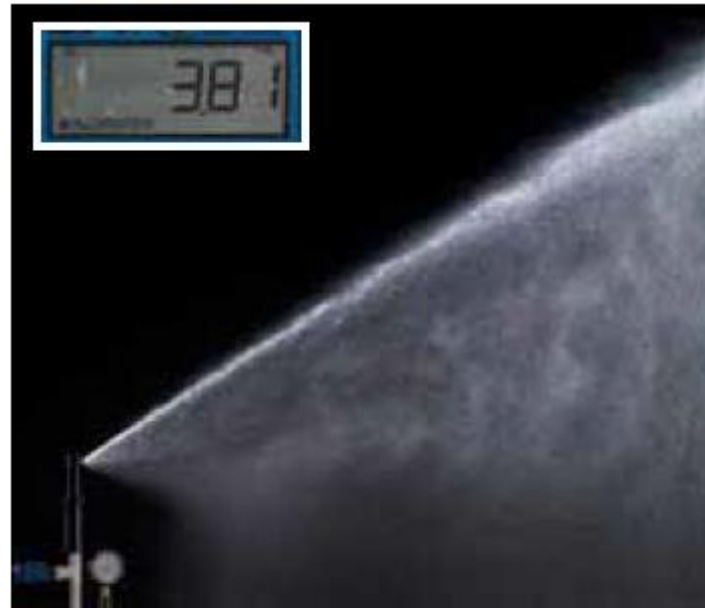
Non-PRS competitive rotor at 79 psi inlet pressure. Without PRS, flow rises to 3.81 gallons per minute.
