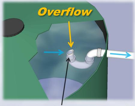
The overflow has a tapered inlet to siphon dust particles off the top surface, and a trap (U-shaped section). It is connected to the storm drain or other approved outlet
